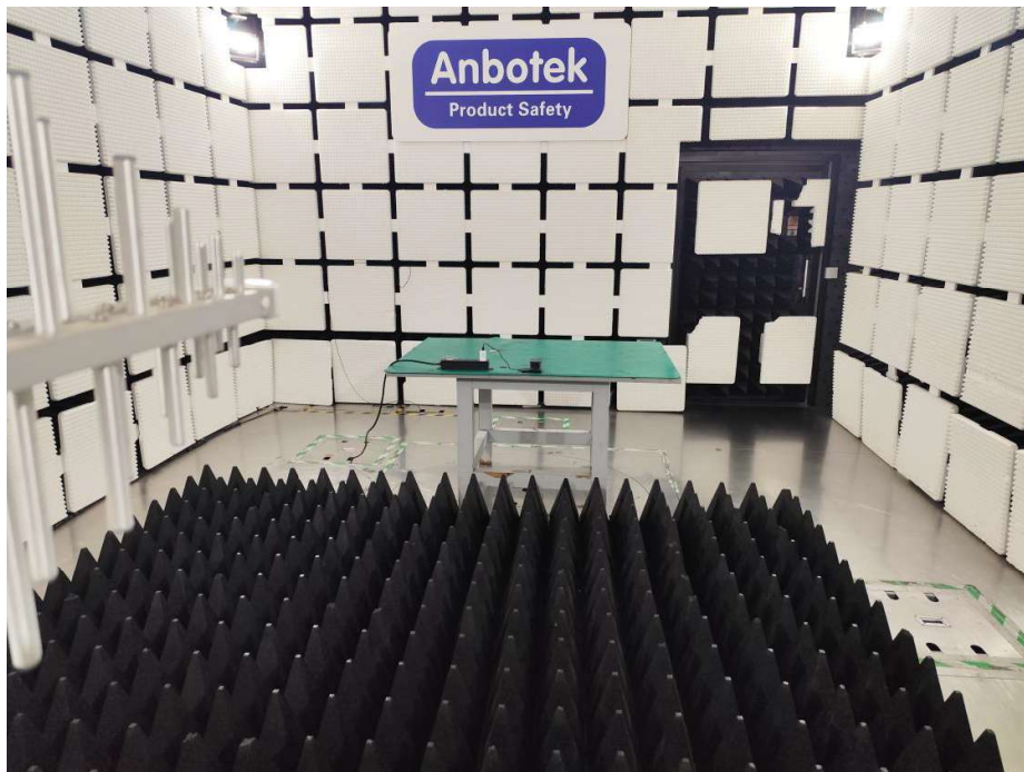
Photo of RF Field Strength Susceptibility Test
