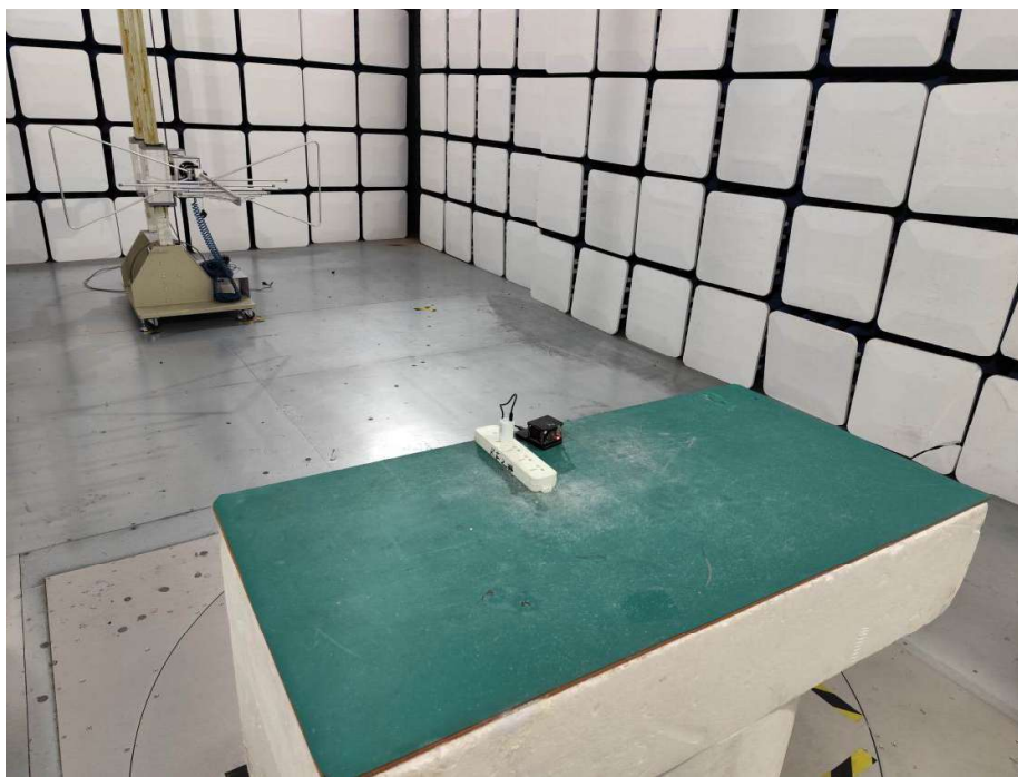
Photo of Radiation Emission Test (Below 1GHz)
